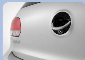
↑Permabond HM162 is used as a threadlocker in this case to secure the rear assist camera mount.
