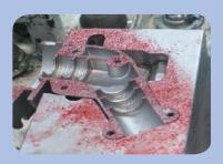
↑Permabond MH196 seals engine castings for lawn equipment. Applied here with a paint roller.
