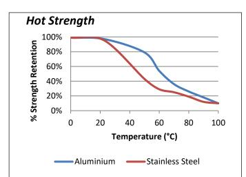
Fully cured specimens conditioned to pull temperature for 30 minutes before testing at temperature.
