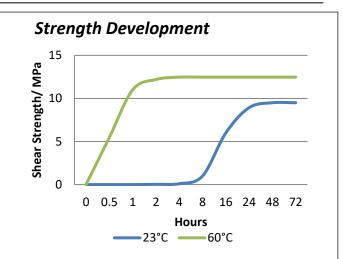
Graph shows typical strength development of bonded aluminium components. Curing at 60°C improves the crosslinking and results in higher final strength values. Lower temperatures will result in a slower cure.
