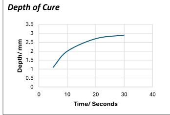
Depth of cure at 25 mW/cm<sup>2</sup> and 405 nm. The depth of cure will depend on the power of the UV lamp, its spectral output, the distance between the lamp and substrates and the transmission characteristics of the substrates.
