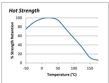
"Hot strength" shear strength tests performed on mild steel. 24-hour cure at room temperature and conditioned to pull temperature for 30 minutes before testing.
