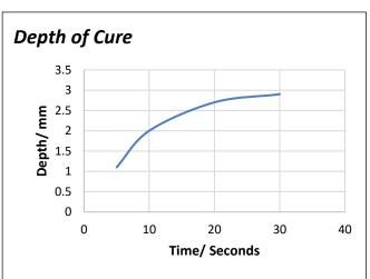
Graph shows the depth of cure at 25 mW/cm<sup>2</sup> and 405nm. The depth of cure will depend on the power of the UV lamp, its spectral output, the distance between the lamp and the adhesive.
