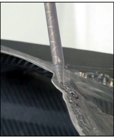
Permabond two part epoxy is used to bond fasteners to a carbon fibre car bonnet and Permabond PT326 bonds the 2 skins of a carbon fibre car bonnet together.
