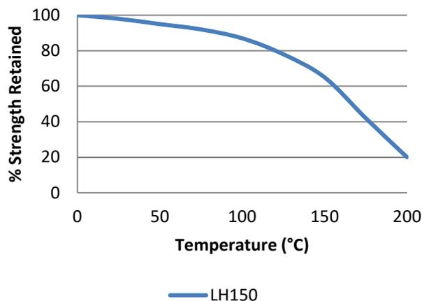
*"Hot strength" Breakaway strength on M10 Zinc plated bolts according to ISO 10964. Cured at 23°C for 24 hours then conditioned for 30 minutes at testing temperature.*
