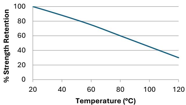
\*\*"Hot strength" shear strength tests performed on mild steel. 24-hour cure at room-temperature and conditioned to pull-temperature for 30 minutes before testing.
