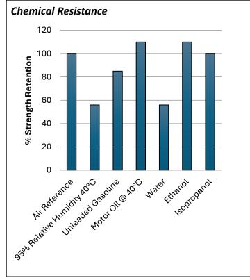
Specimens were immersed for 1000 hours at 22°C (unless otherwise stated).
