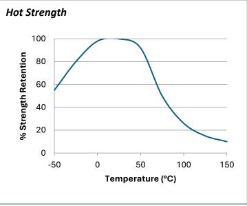
\*"Hot strength" shear strength tests performed on mild steel.
